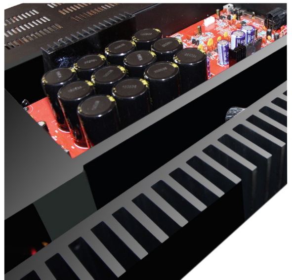
Large heatsink and 12 10,000 \mu F each, or 120,000 \mu F.
